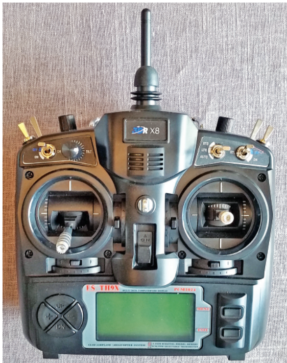
A drone controller with a twist knob potentiometer at the upper left that controls the EPM (similar to a camera gimbal control).
