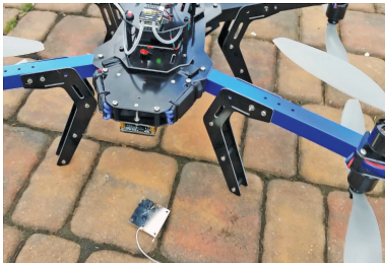
A mounting plate for an EPM, which is visible at the very front of the drone.
