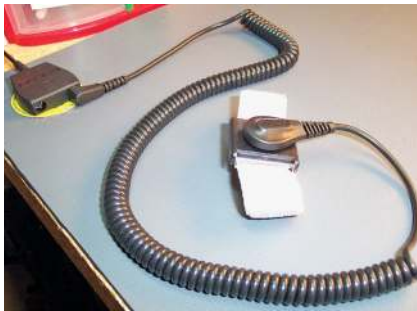
Figure 2 — The wristband, which plugs into the antistatic mat's ground connection point.
