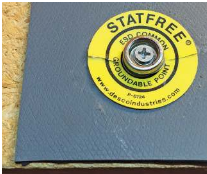
Figure 3 — The antistatic mat ground connection point.
